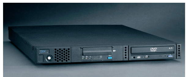
IBM 7212 1U Dual Bay Enclosure
